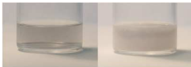
Figure 1. Thermomorphic behavior of dendritic nanocarrier 9 in FC-75 in the presence of encapsulated bromophenol blue: left, 70°C (clear solution); and right, 20°C (suspension).
